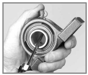
**Figure 56.** Bearing positioning for removal.
